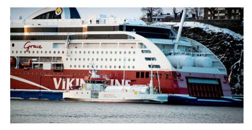
Fig. 6.2. Viking Grace in the Port of Stockholm – ship to ship bunkering operation
