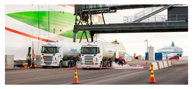
Fig. 6.1. LNG bunkering in the Port of Helsinki (Megastar ferry)
