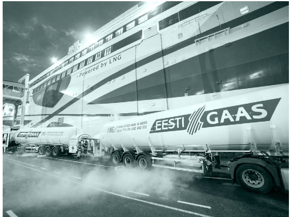
FIGURE 11 TTS bunkering of M/S Megastar Source: Ports of Tallinn
