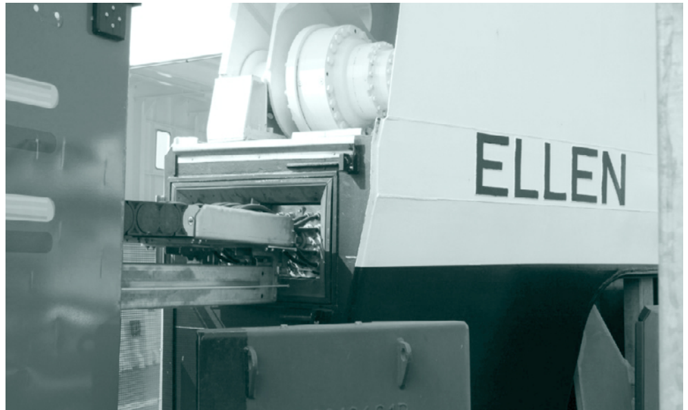
FIGURE 38 Mobimar shore-side charging cable connector in Søby harbour Photo by Halfdan Abrahamse
