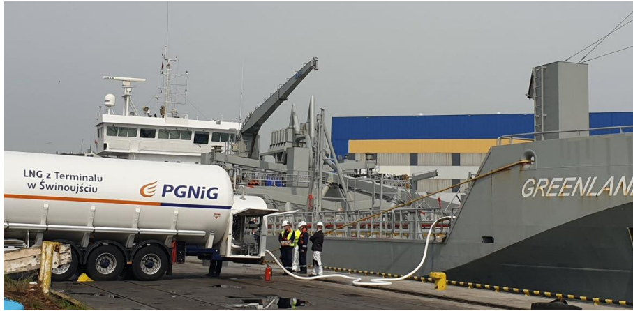
LNG Bunkering truck to ship in Port of Gdynia
